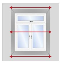
2. Measure the Height in at least 3 different places. Remember to include the space needed on the wall or architrave for each side of the shutter frame. Note the smallest dimension you find and add 46mm in height. This is the deduction applied and now the spec can be submitted
