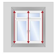
Important: Remember to measure the recess where you plan to fit the frame
