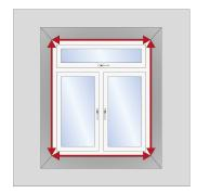
A recess is the space created when a window is set back from the interior wall of the room. A reveal fix involves installing the shutter within that recessed opening
