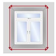
A non-recess window is not set back from the interior wall. If there is no recess, the shutters will need to be outside mount fixed/face fixed – they can be attached to the window frame, trim, or surrounding walls.
